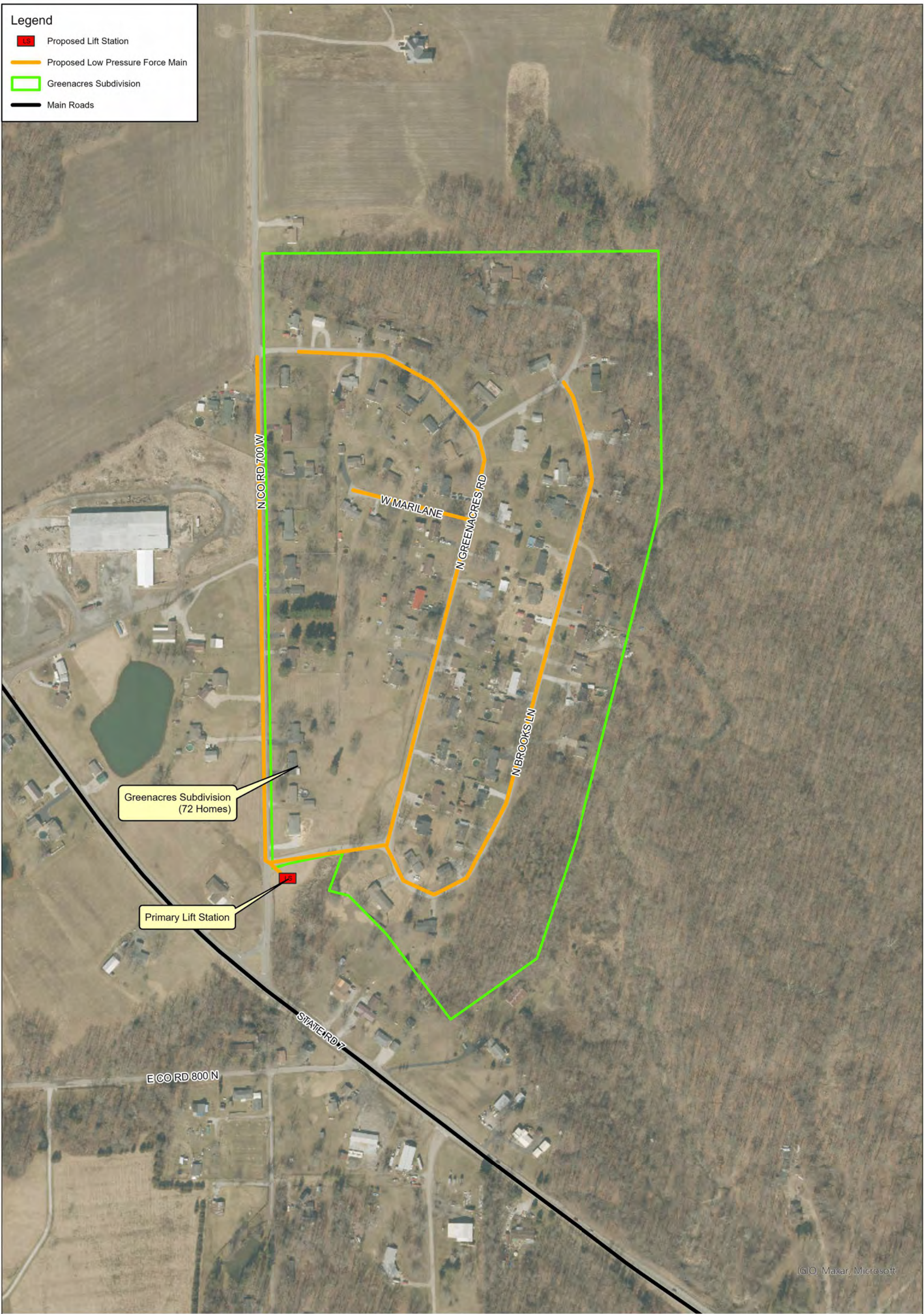
Figure 4.3a Jennings County Sanitary Master Plan Greenacres Subdivision Alternative #3 Low Pressure Sewer with Grinder Pumps Jennings County, Indiana
